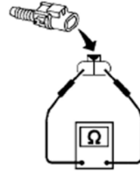
Figure 13 : Testing the Elements.
