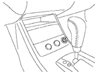
Figure 10 : Typical Switch Mounting Location.
